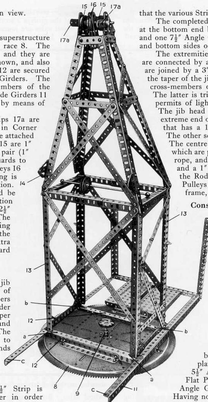
Fig. 4. The Superstructure and upper Slewing Race
