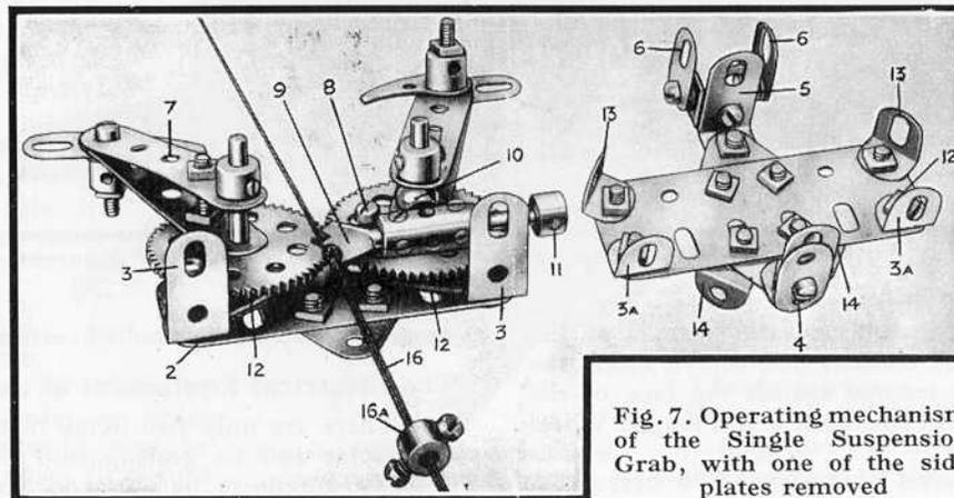
Fig. 7. Operating mechanism of the Single Suspension Grab, with one of the side plates removed
