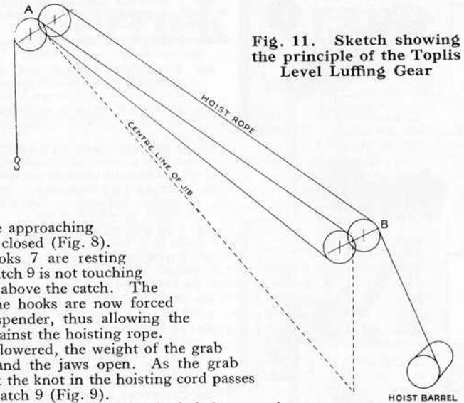
Fig. 11. Sketch showing the principle of the Toplis Level Luffing Gear
